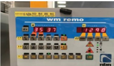
Water mixer system upgrade Shortening recirculation cycles of conventional mixing systems, resulting in water and energy savings
